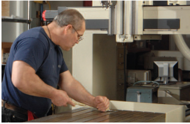
Hand scraping to ensure new machine tolerances
